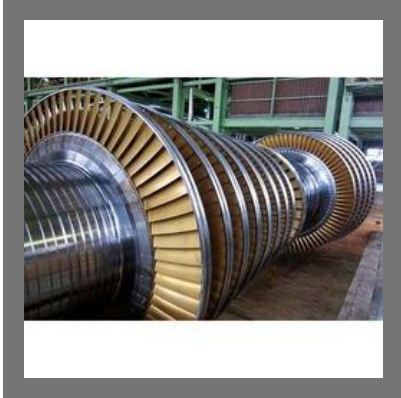
Multi Stage Steam Turbine
