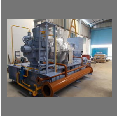
MW Steam Turbine
